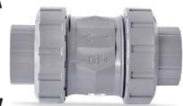
Check Valve type 562 CPVC SF With Solvent cement sockets Inch ASTM
